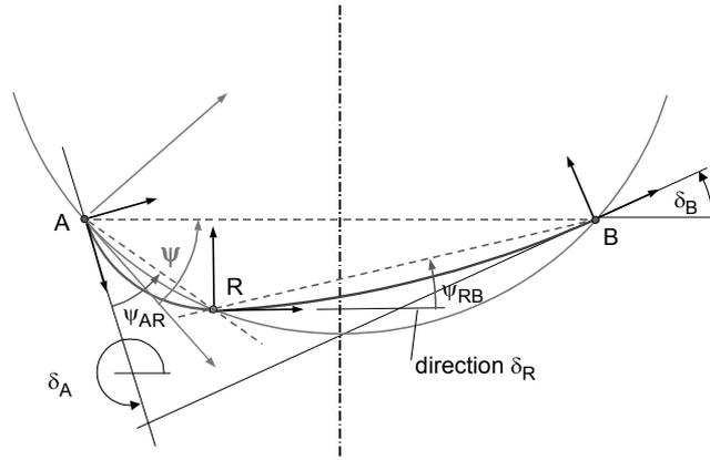
Fig. 8 Connection point R of the two arcs on the circle of Struycken
