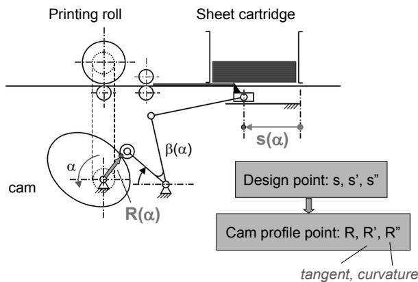
Fig. 3 Cam profile information as available from the design: discrete points and derivatives
