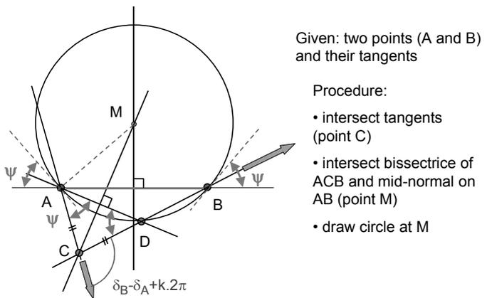
Fig. 6 Geometric construction of the circle, which is the locus of connection points between two arcs (acc. Struycken)
