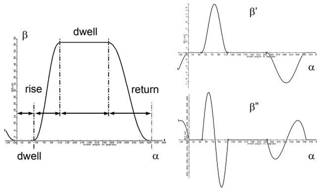
Fig.2 Typical motion definition with continuous functions
