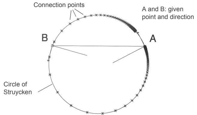
Fig. 5 Connection points between the two arcs when the curvature of one arc will be varied
