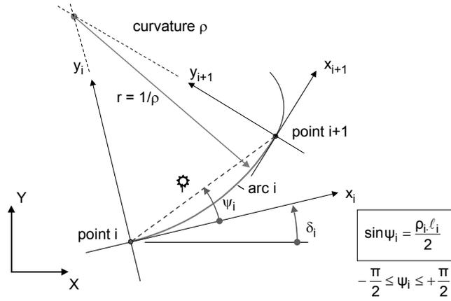
Fig. 7 Special definition of the arc in local co-ordinate system
