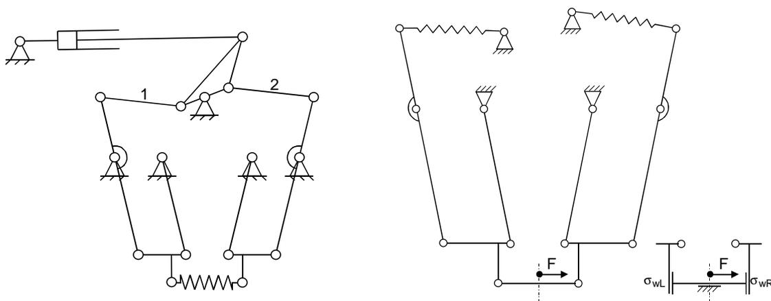
Fig. 6 Mechanism model for analysis of force amplification (left) and compliance (right)
