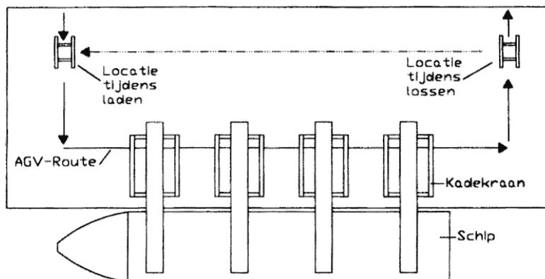
Fig. 1 Typical terminal layout
