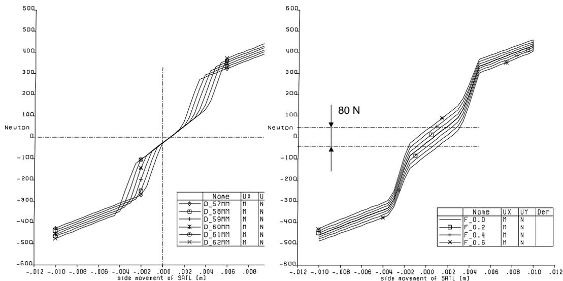
Fig. 9 Compliance characteristic without friction      Fig. 10 Compliance characteristic with friction
