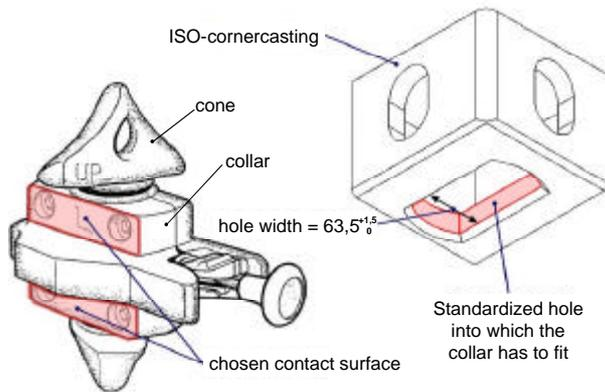
Fig. 2 Example of a semi-automatic twist-lock
