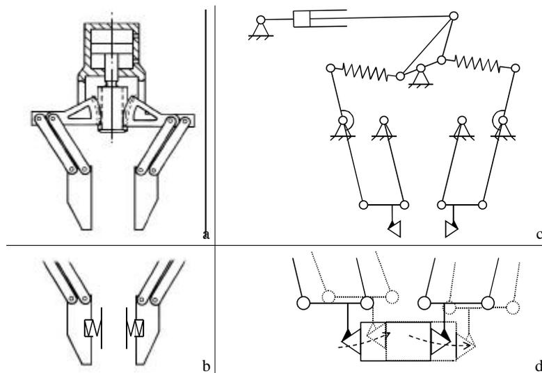
Fig. 5 Parallel jaw grippers
