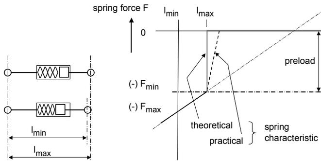
Figure 7 Characteristic of preloaded spring
