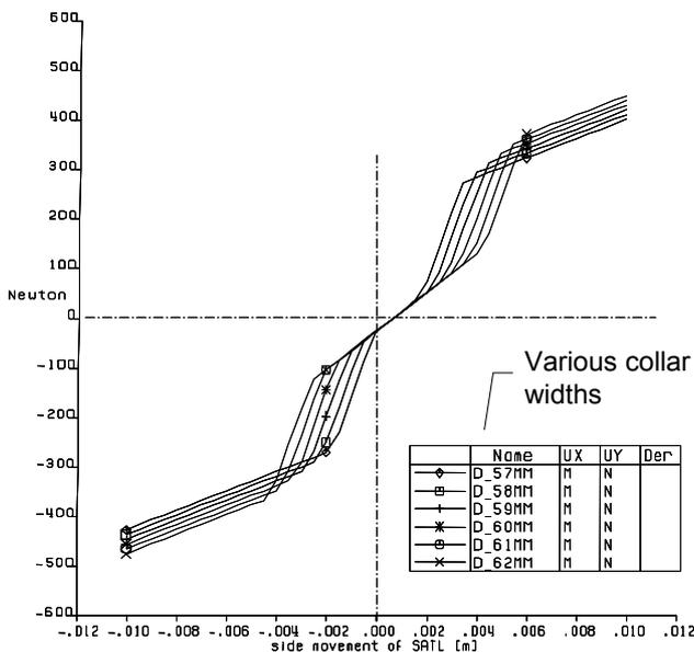
Figure 8 Compliance characteristic without friction
