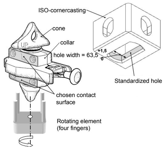
Figure 2 Semi-automatic twist-lock
