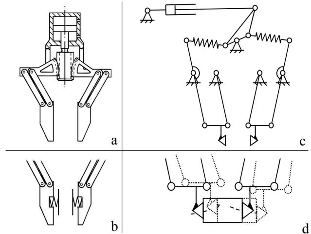
**Figure 5 Parallel gripper configurations**
