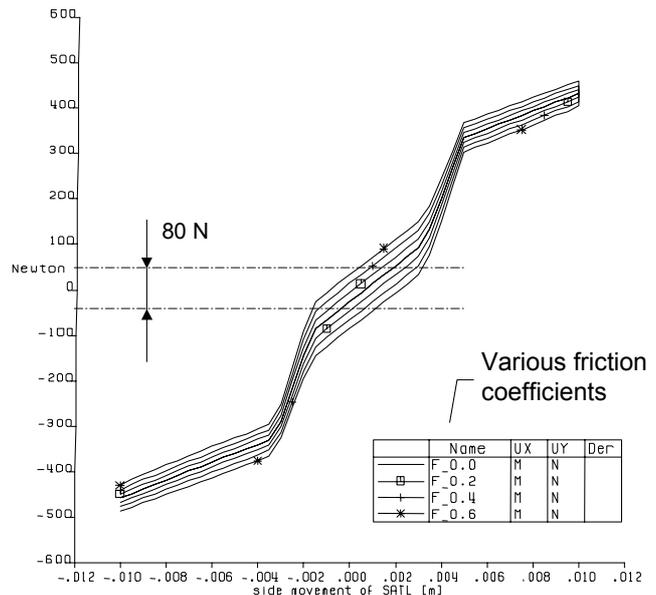
Figure 9 Compliance characteristic with friction (twist-lock width 60 mm)
