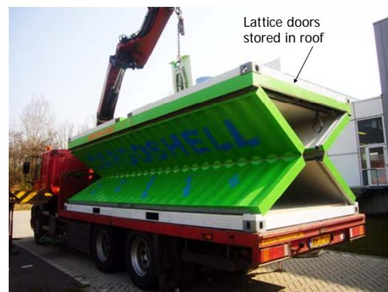
Fig. 13 Cargoshell foldable container
