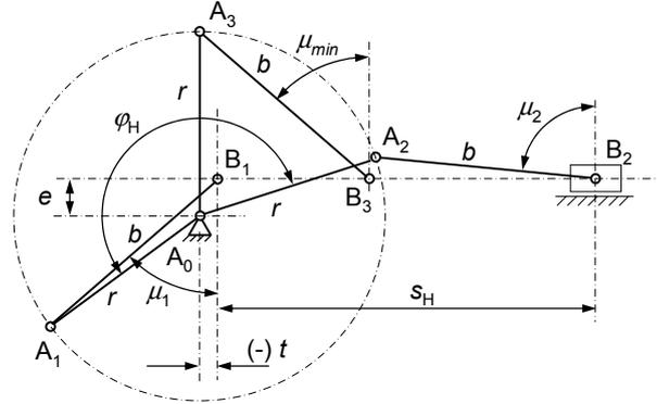
Fig. 1 Crank-slider mechanism in the three design positions
